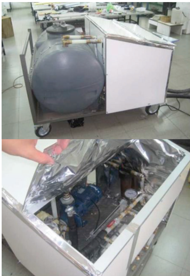
Figure 8: TRT equipment built for this research
