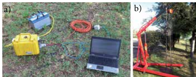
Figure 3: MASW field setup, a) seismograph, laptop and peripherals and b) impact load
